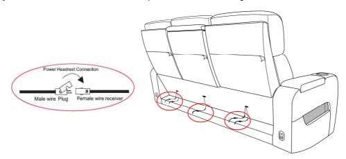
**Step 4:** Latch male wire plugs from middle backrest (reading lights) to female wire receivers located at the bottom back underneath the flap.
