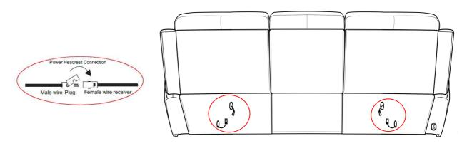
**Step 4:** Connect wall plug transformer to transformer switch. And connect transformer plug to electrical outlet.
