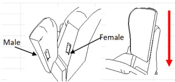
**Step 3:** Attach the LSF wing and RSF wing by inserting the male KD brackets into the slot of the female brackets, pressing firmly downward until
