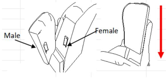
**Step 4:** Attach the LSF wing and RSF wing by inserting the male KD brackets into the slot of the female brackets, pressing firmly downward until
