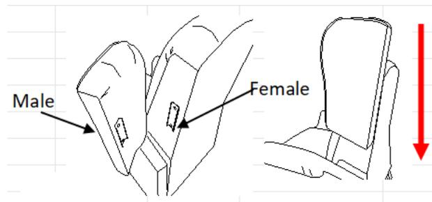
**Step 2:** Attach the LSF wing and RSF wing by inserting the male KD brackets into the slot of the female brackets, pressing firmly downward until
