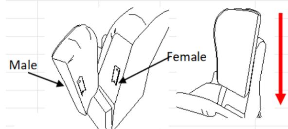
**Step 4:** Attach the LSF wing and RSF wing by inserting the male KD brackets into the slot of the female brackets, pressing firmly downward until
