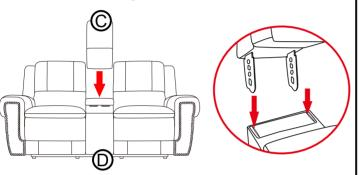
Step2 Position the Backs(A/B) with clips on over the mechanism tab at rear of Body(D) as picture below. Ensure both clips on back are aligned with tabs, then press top of back frame downward until **a clicking sound is heard**.
