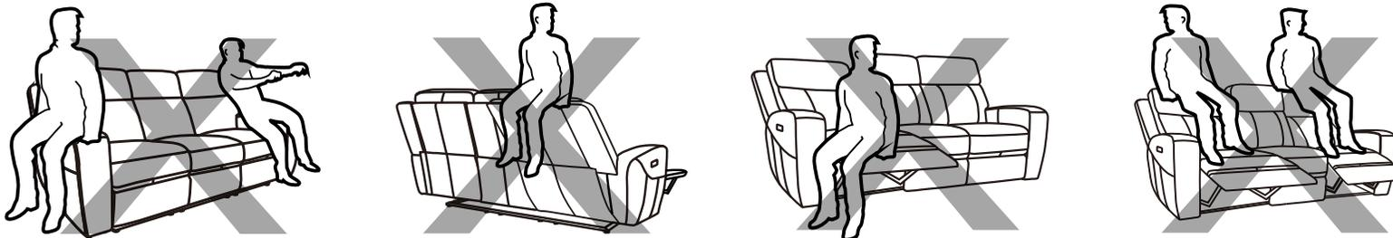
\*If unit must be moved, do not drag. Unit must be lifted in order to be moved.
