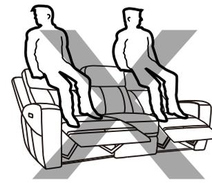
\*If unit must be moved, do not drag. Unit must be lifted in order to be moved.
