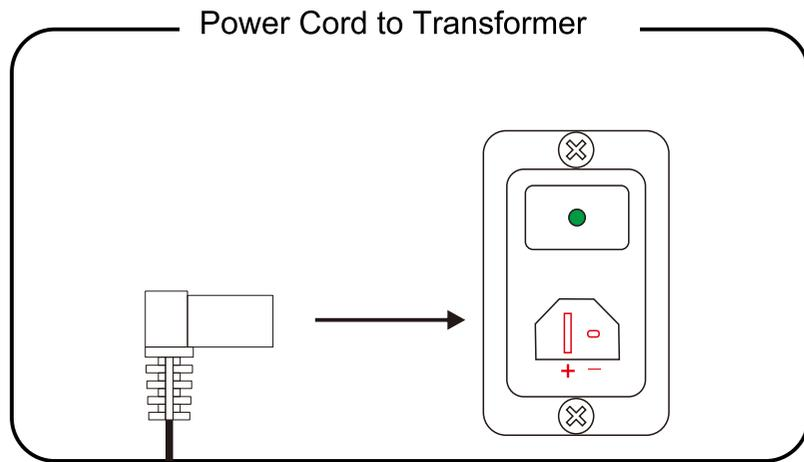
STEP 5: Connect wall plug transformer to outlet.
