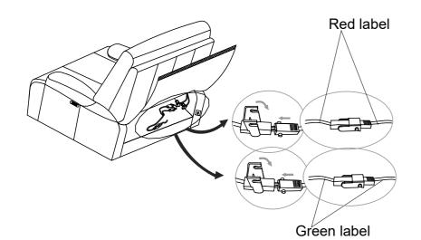
Step 5: Connect wall plug transformer to transformer switch. And connect transformer plug to electrical outlet.
