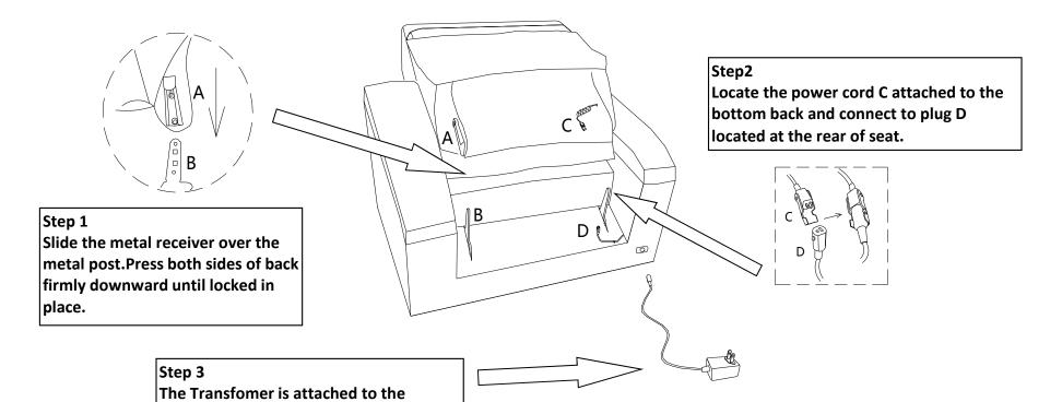
**Note:** Make sure all PLUGS are connected on the product before plugging power cord into power outlet. If not damage can occur.
