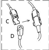
**Note:** Make sure all PLUGS are connected on the product before plugging power cord into power outlet. If not damage can occur.
