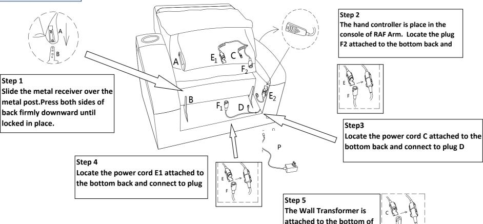
**Note:** Make sure all PLUGS are connected on the product before plugging power cord into power outlet. If not damage can occur.
