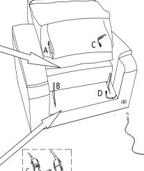
Step 3 Locate the transfomer, which is is attached to the bottom of the rail. Connect the transformer to the DC Port, which is located at the rear of arm.
