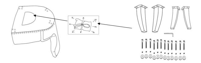
Step 2:Insert the front leg (A&B) and back leg (C&D) to seat frame by using flat washer (F), spring washer (H), bolt (G). Then tighten the bolts with allen wrench (E).
