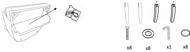
Step 2: Insert the front legs(P2) and back legs (P3)into the Seat (P1) bottom, Lock legs by using Flat washers (H2) and spring washer(H4) and bolts (H1). Then tighten the bolts with allen wrench (H3).
