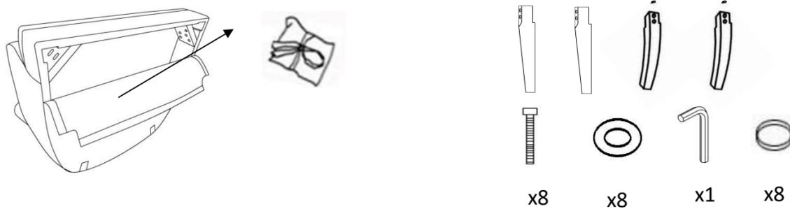
Step 2: Insert the front legs(P2) and back legs (P3)into the Seat (P1) bottom, Lock legs by using Flat washers (H2) and spring washer(H4) and bolts (H1). Then tighten the bolts with allen wrench (H3).
