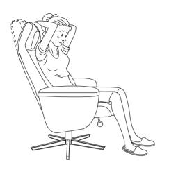
To adjust the headrest, grip the backside of the headrest and pull forward from both sides as shown
