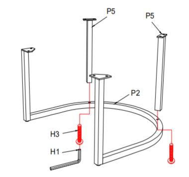
Step 3.Attach assembled U-shaped Support Bar(P2) to Chair Top(P1) with bolt(H2),tigh wrench(H1) as illustration below.
