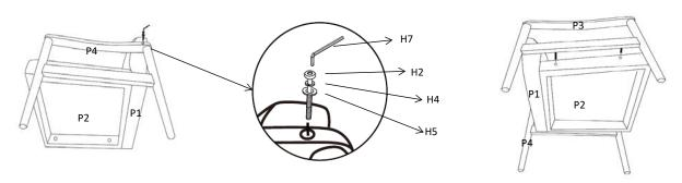
Step 6.Insert the flat washer(H6), lock washers(H4) and nuts(H3) to the end of stud(H1) to assembly the armrests(P3&P4) to seat backrest(P1&P2). Tighten all the nuts(H3) by spanner(H8).
