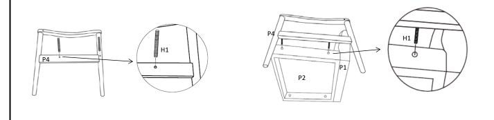
Step 5.Insert the flat washer(H5), lock washers(H4) and bolts(H2) to the right armrest(P4). Securely tighten all bolts with Allen wrench (H7) in right way. Use the same Step 4 and Step 5 to assembly the left armrest(P3) to seat backrest(P1&P2).
