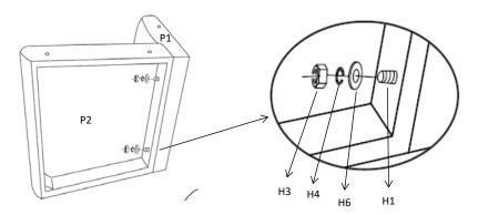
Step 4.Screw the studs(H1) into the hole in right armrest(P4),make sure all the studs(H1) were fully tightened. Then insert the studs(H1) in right armrest(P4) into the hole of the seat backrest(P1&P2) as shown.
