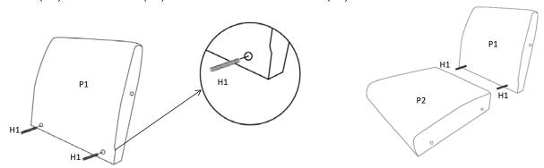
Step 3. Open the black fabric on bottom. Insert the flat washer(H6), lock washers(H4) and nuts(H3) to the end of stud(H1) to assembly the backrest(P1) to chair seat(P2). All the nuts(H3) by spanner(H8).(NOTE: Don't fully tighten the nuts.)
