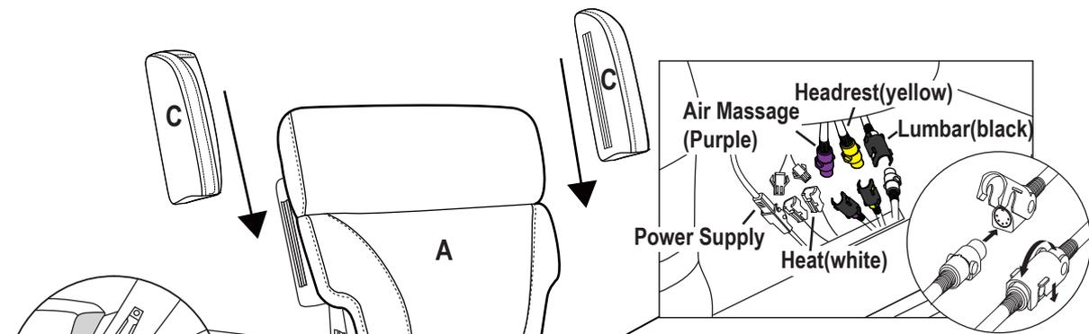
Ensure both clips on back are aligned, then press top of back frame downward until a clicking sound is heard.
