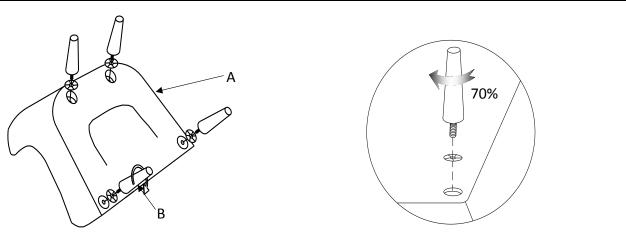
1 Put Chair Body(A) on a non-abrasive table. Insert Legs(B) into the back of Chair Body(A), and assemble using four plastic washers(1)to screw in. Do not fully tighten any leg. Tighten to about 70% of full insertion
