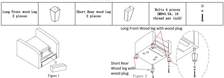
1. The Wooden Legs are located at the rear of seat cushion, remove all the Wooden Legs from the box(See Figure 1). Attach each wooden leg to its corresponding pre-drilled hole by turning in a clockwise direction until secure (this can be done by hand(See Figure 2).
