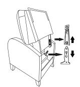
**3**. To remove the back, lift the tab on both sides and pull the back straight up. Note: if there is difficulty in getting the back to lock into place check to see that the tab is engaged in the proper space.
