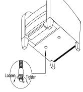
Note: There are no tension adjusters on mechanisms #1632, #1671, #1672, #2032, #2034, or #2072. But mechanisms #8550, #2000, 7550 or #8546 have the tension adjusters and you can get the mechanism numbers from the side of the mechanism. Follow point 5 above to adjust the tension.
