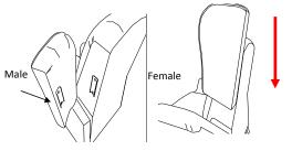
**5**. KD Wings(If applicable) Insert the male KD Bracket into the slot of the female Bracket pressing firmly downward until the frame is tight.
