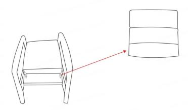
Install the Backrest into the Seat by positioning female metal receiver brackets over male metal posts.
