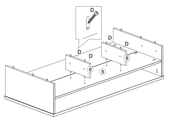
Fix the part (6) to the part (5) using the screw (D)
