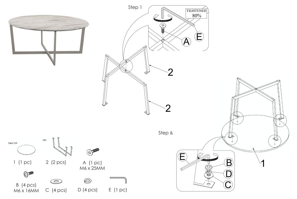
During assembly, hand tighten screws only. When all screws are in place, then tighten completely.
