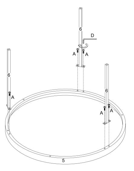
Using bolt (A) attach part (6) into part (5) with hex key (D) as per diagram.
