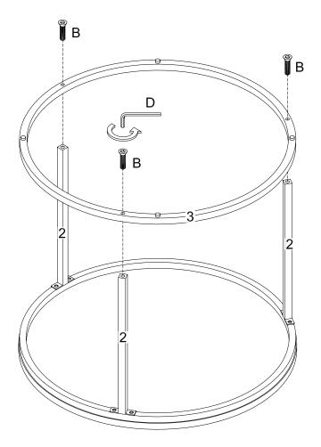
Using bolt (B) attach part (3) into part (2) with hex key (D) as per diagram.
