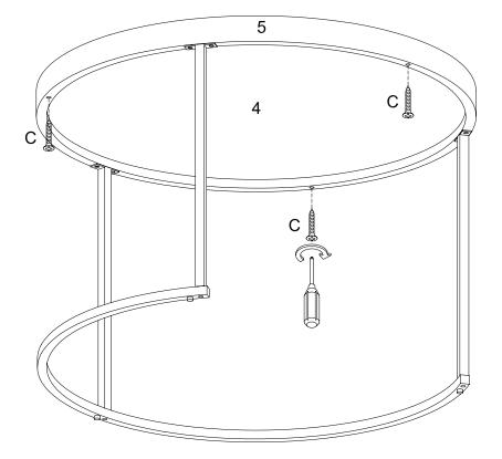
Using screw (C) secure part (4) into part (5) with Philips head screwdriver as per diagram.
