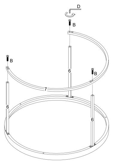
Using bolt (B) attach part (7) into part (6) with hex key (D) as per diagram.
