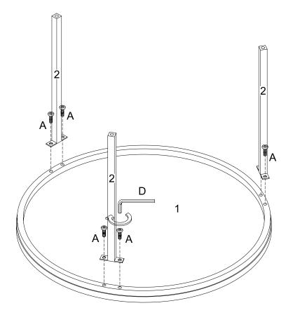
Using bolt (A) attach part (2) into part (1) with hex key (D) as per diagram.
