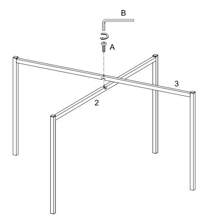
Use wrench (B), to secure legs (2,3) with bolt (A).
