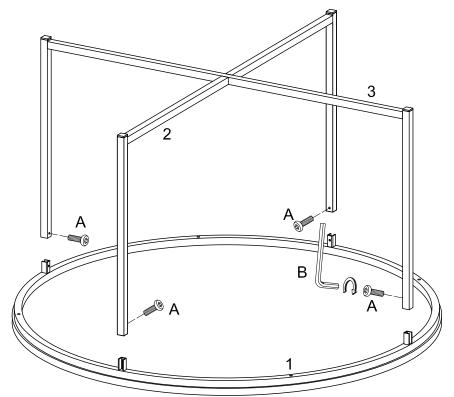
Use wrench (B), to secure legs (2,3) to table top (1) with bolts (A).
