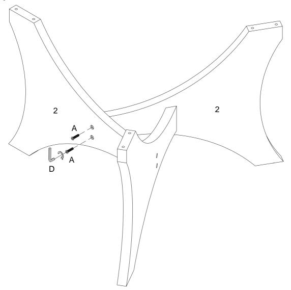
Using bolt (A) attach part (2) to part (2) with Hex key (D) as per diagram.
