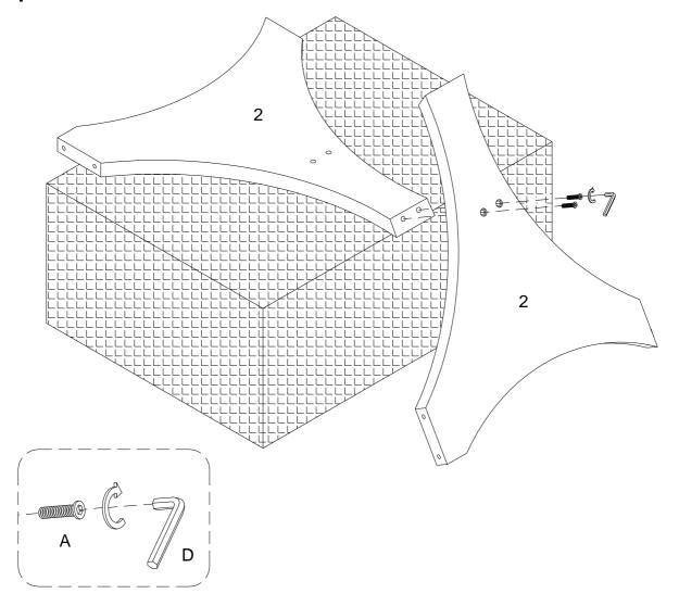
Using bolt (A) attach part (2) to part (2) with Hex key (D) as per diagram.
