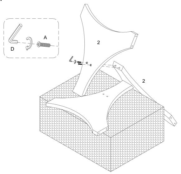
Using bolt (A) attach part (2) to part (2) with Hex key (D) as per diagram.
