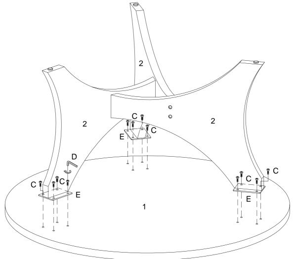
Using bolt (C) attach Plate (E) to part (1) with Hex key (D) as per diagram.
