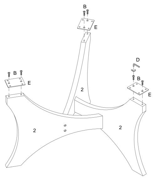
Using bolt (B) attach Plate (E) to part (2) with Hex key (D) as per diagram.
