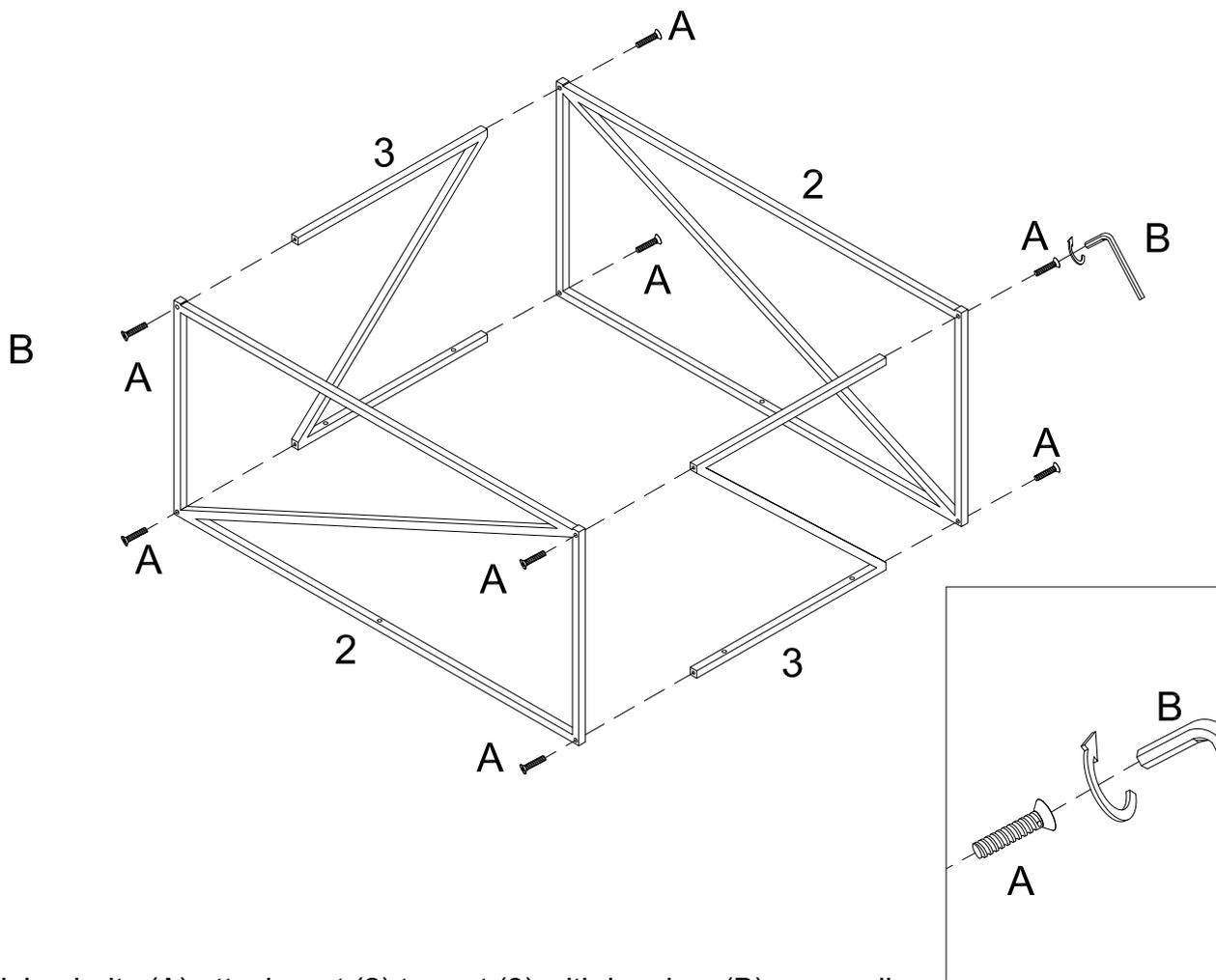
Using bolts (A) attach part (2) to part (3) with hex key (B) as per diagram.
