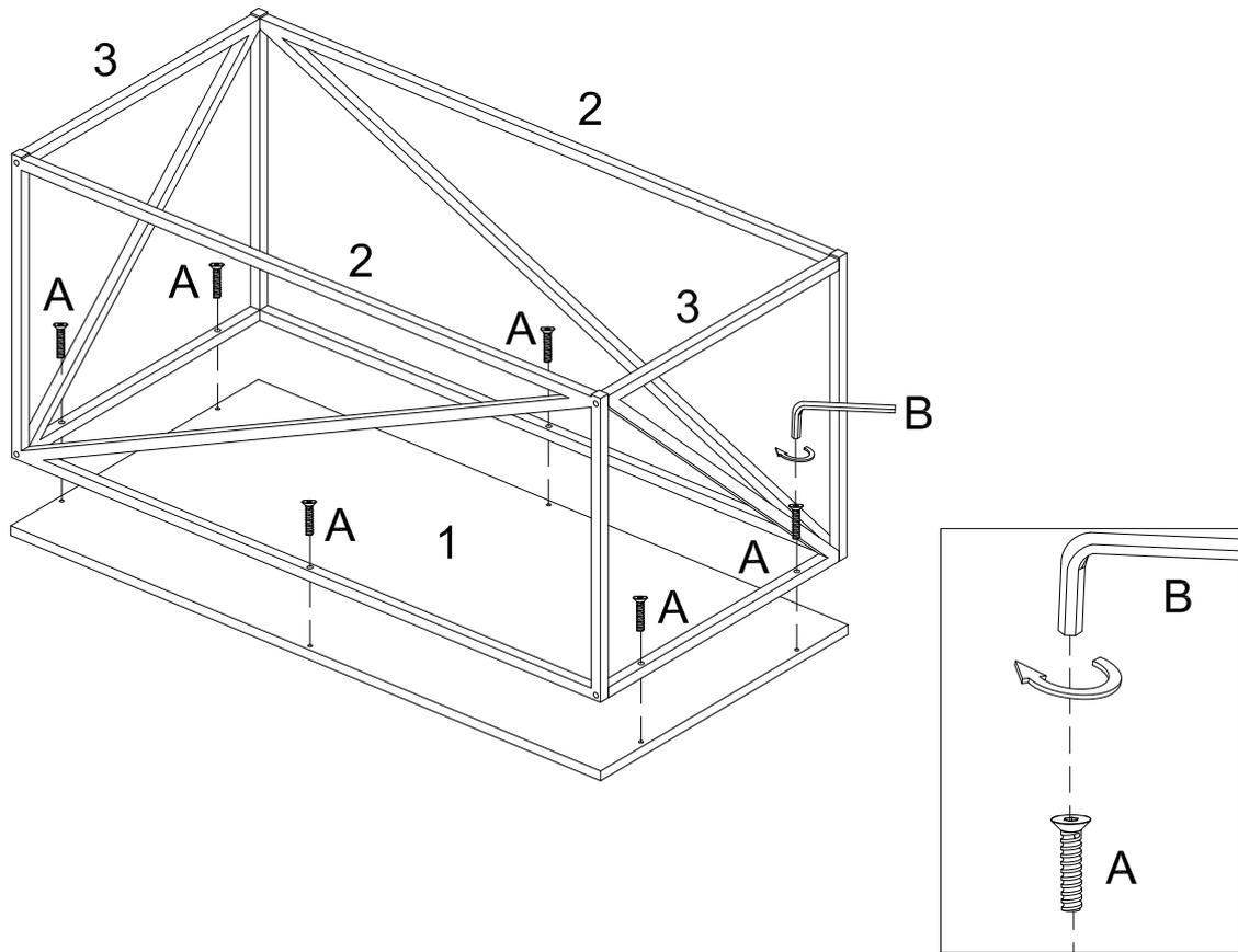
Using bolts (A) attach parts (2,3) to part (1) with hex key (B) as per diagram. Then fully tighten all the bolts.
