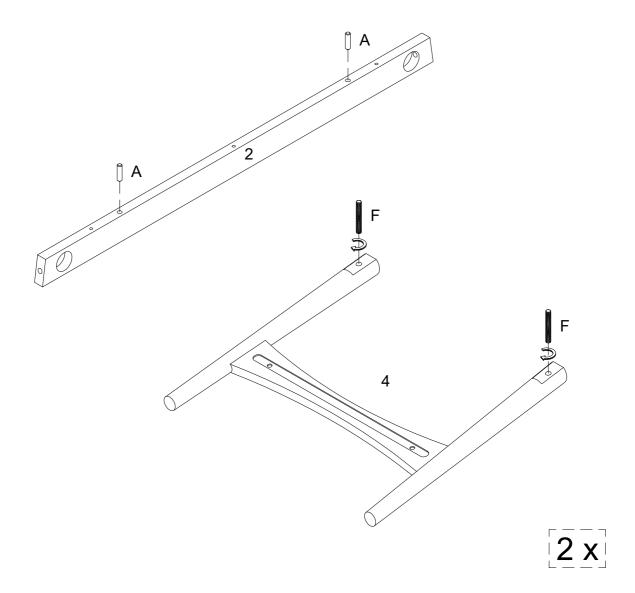
Insert wooden dowel (A) into part (2) and secure bolt (F) into part (4) as per diagram.
