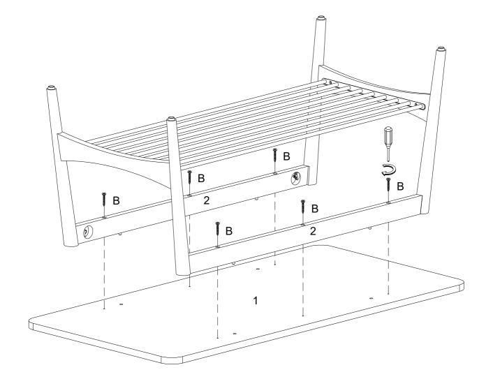
Using Flat head screw(B) secure part (2) to part (1) with Philips head screwdriver as per diagram. Note: Fully tighten all bolts.
