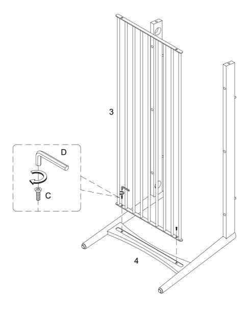
Using bolt (C) attach part (3) to part (4) with Hex key (D) as per diagram. Note:Do not fully tighten all bolts.
