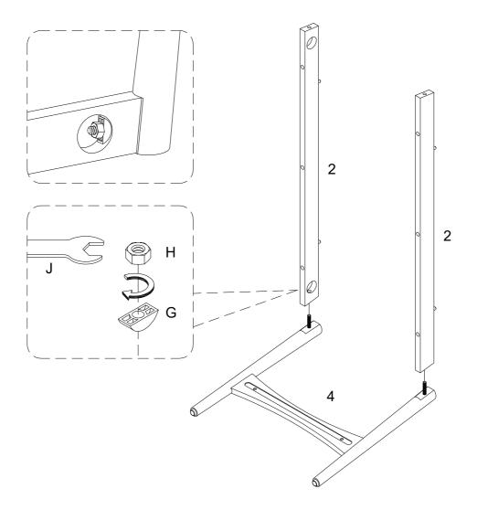
Using washer (G) and Nut (H) secure part (2) into part (4) with Wrench (J) as per diagram.
