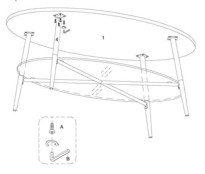
Using bolt (A) attach part (4) to part (1) with Hex key (B) as per diagram. Note: Fully tighten all bolts at this step .
