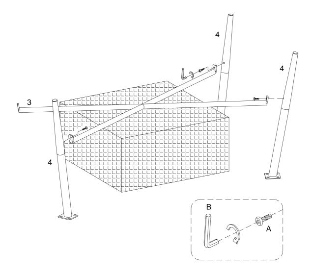
Using bolt (A) attach part (3) to part (4) with Hex key (B) as per diagram. Note: Please do not fully tighten all bolts at this step .
