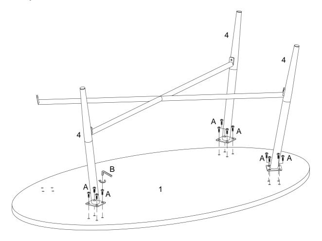
Using bolt (A) attach part (4) to part (1) with Hex key (B) as per diagram.
