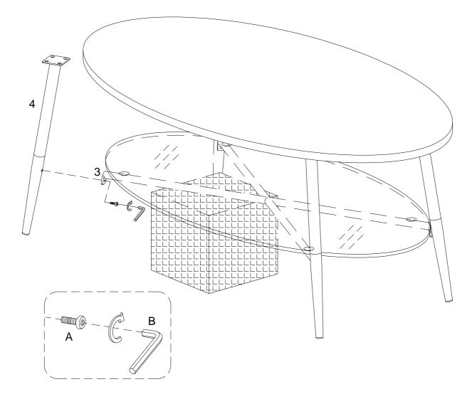
Using bolt (A) attach part (3) to part (4) with Hex key (B) as per diagram.
