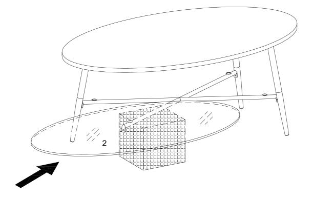
Place part (2) on the top of part (3) carefully as per diagram.
