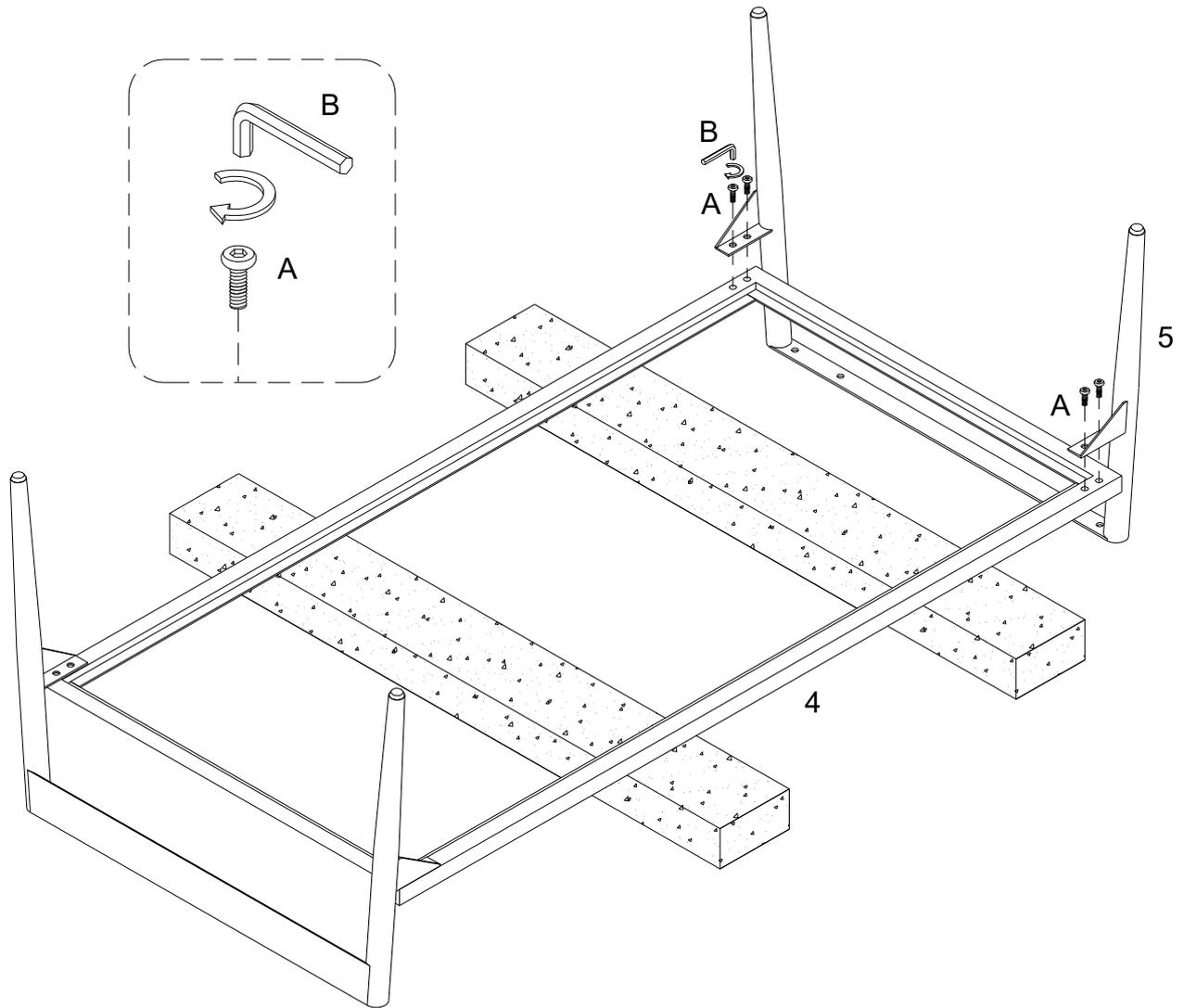
Using bolt (A) secure part (5) to part (4) with hex key (B) as per diagram.
