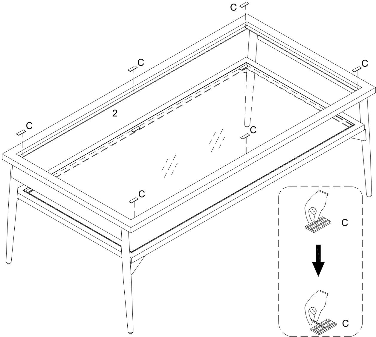
Tear off glass pad (C) and place it on part (2) as per diagram.
