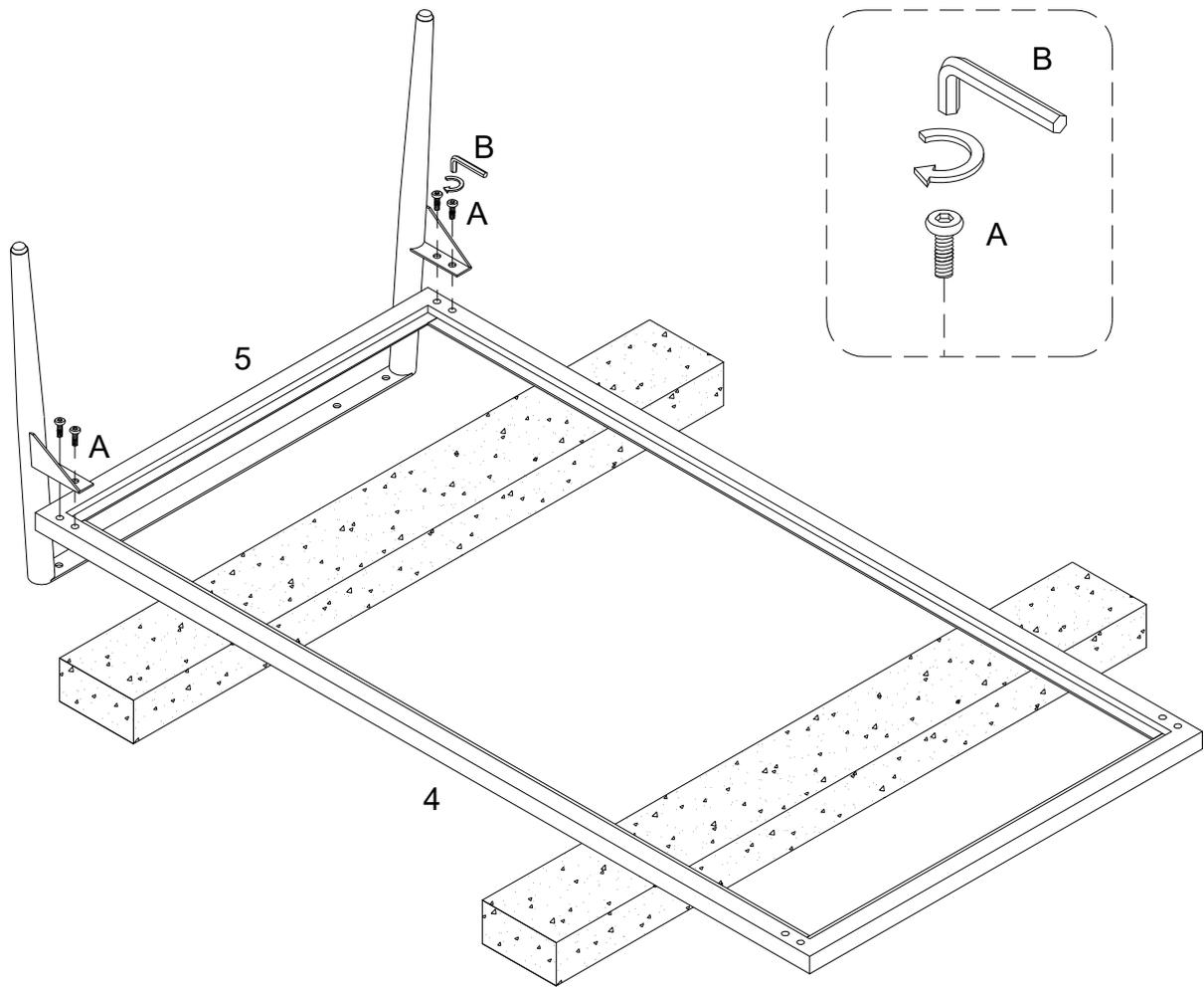
Using bolt (A) secure part (5) to part (4) with hex key (B) as per diagram.
