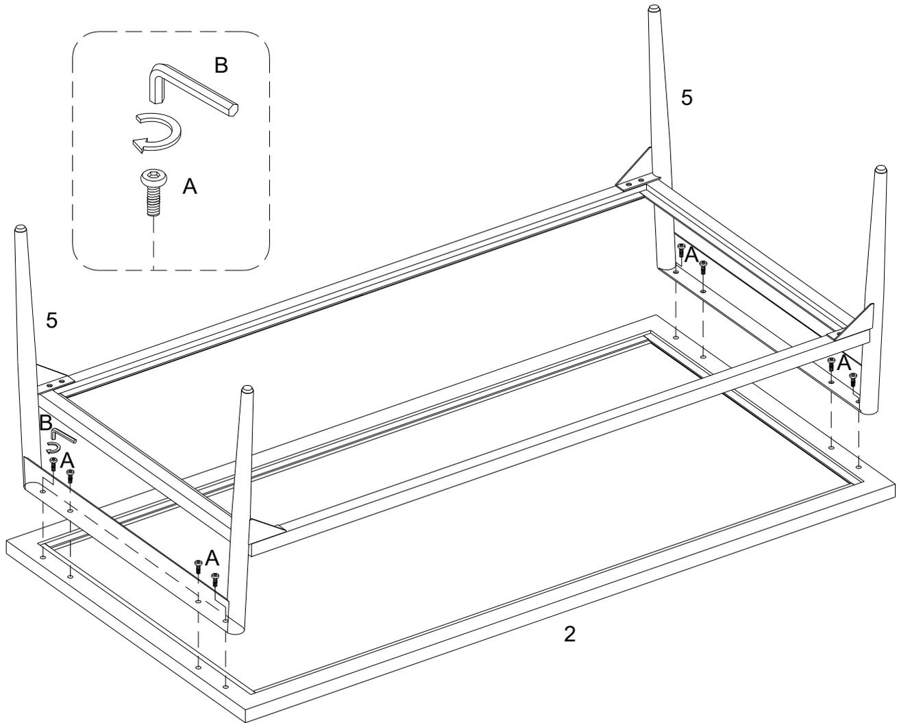
Using bolt (A) secure part (5) to part (2) with hex key (B) as per diagram.
