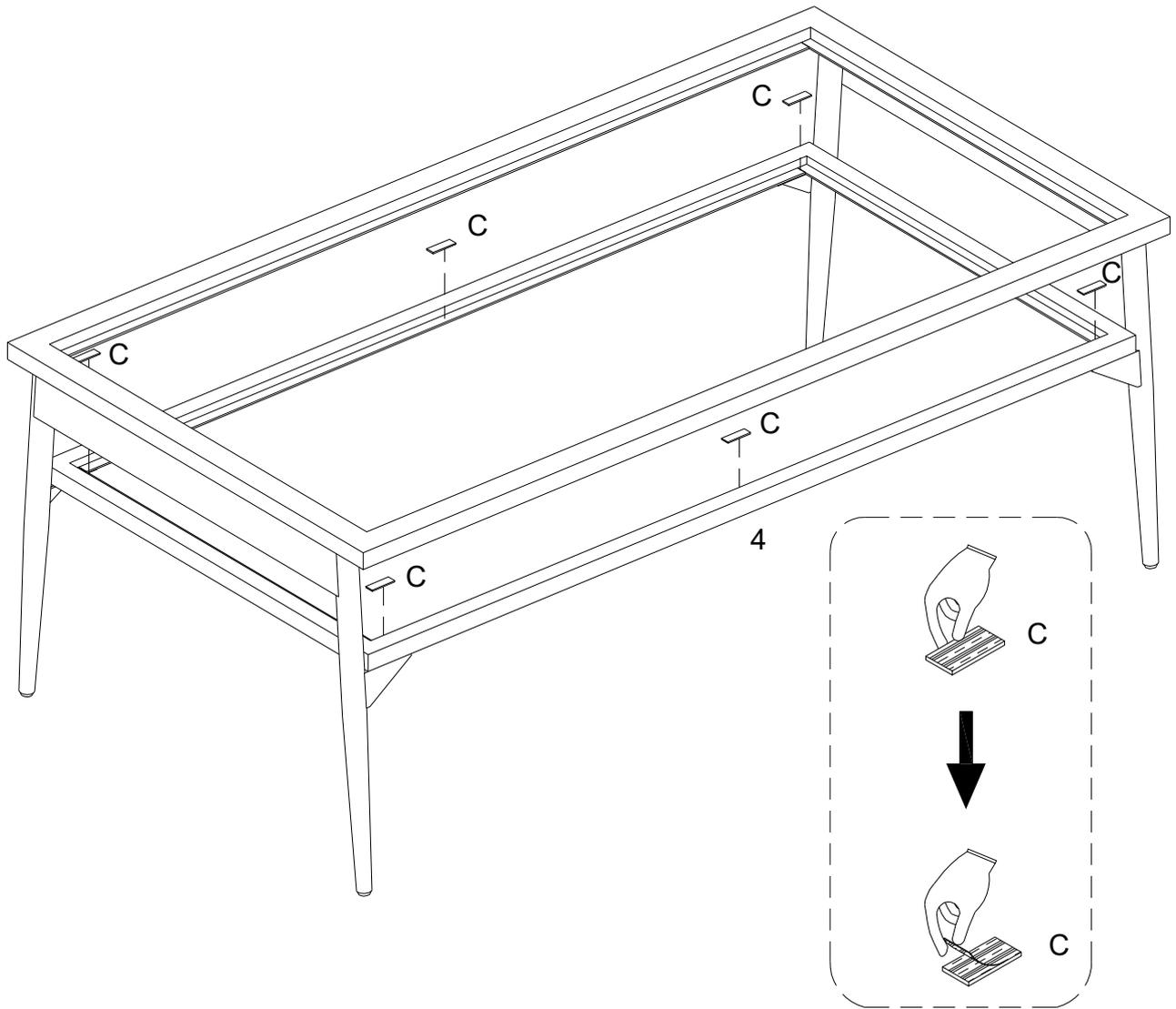
Tear off glass pad (C) and place it on part (4) as per diagram.
