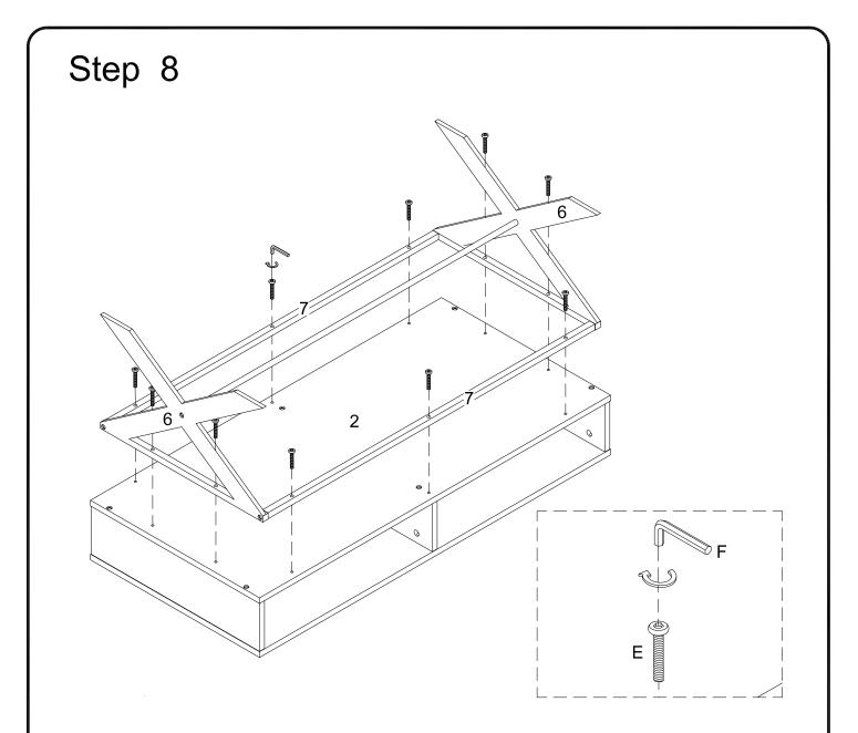
Using bolt (E) attach parts (6,7) to part (2) with hex key (F) as per diagram. Fully tighten all the bolts.
