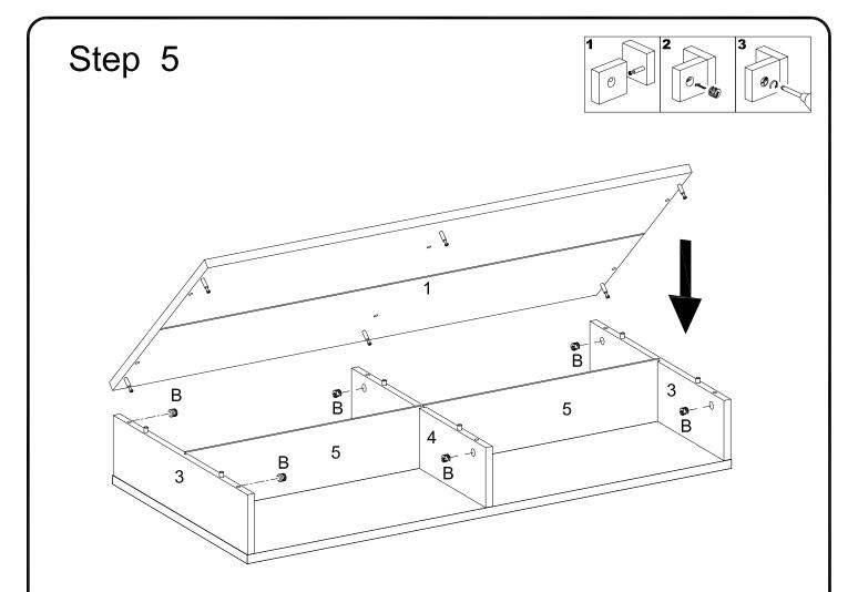
Using cam lock(B) secure part (1) to parts (3,4) with Philips head screwdriver as per diagram.
