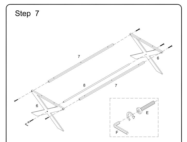
Using bolt (E) attach parts (7,8) to part (6) with hex key (F) as per diagram. Do not fully tighten all the bolts.
