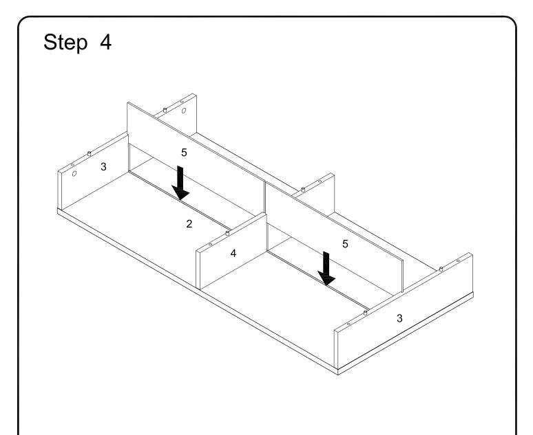
Put part (5) into parts (2,3,4) as per diagram.
