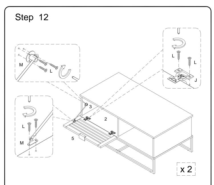
Using screw (L) secure Europe hinge (J) into parts (2), then using screw (L) secure door hinge (M) into parts (3,5) with Philip head screwdriver as per diagram.
