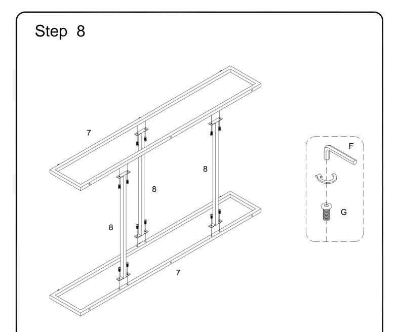
Using bolt (G) secure part (8) into part (7) with hex key (F) as per diagram. Do not tighten all the bolts .
