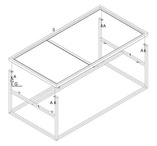
Using bolt (A) attach part (1) to part (3) with Hex key (G) as per diagram.
