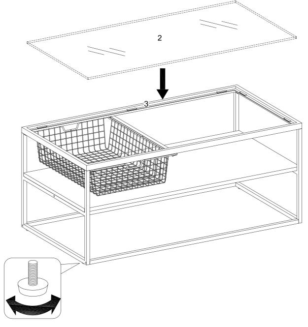
Put part (2) to part (3) carefully as per diagram.
