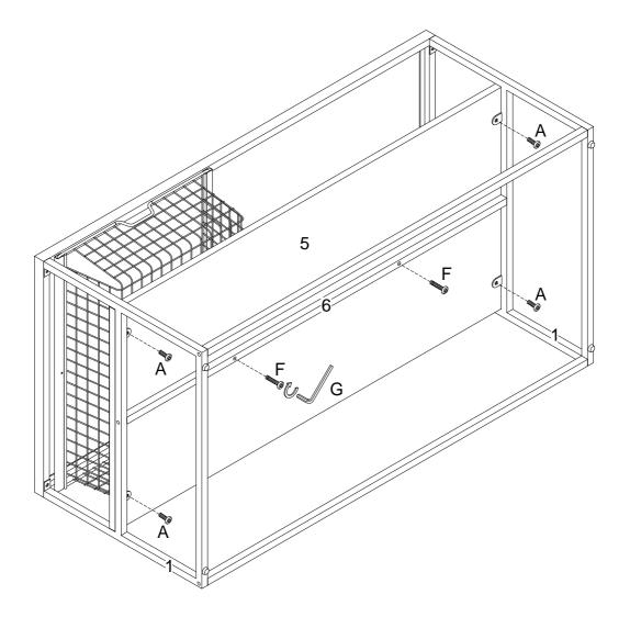
using bolt (A) secure part (1) to part (5),then using bolt (F) secure part (6) to part (5) with Hex key (G) as per diagram.
