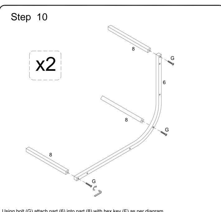
Using bolt (G) attach part (6) into part (8) with hex key (F) as per diagram.
