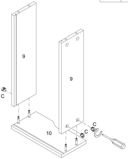
Using cam lock(C) attach part (9) to part (10) with Philips head screwdriver as per diagram.
