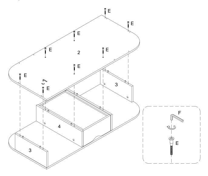
Using bolt (E) attach part (2) into parts (3,4) with hex key (F) as per diagram.
