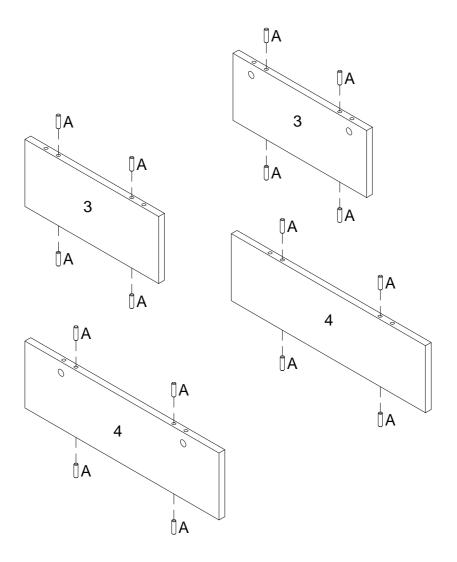
Insert wooden dowel (A) into parts (3,4) as per diagram.
