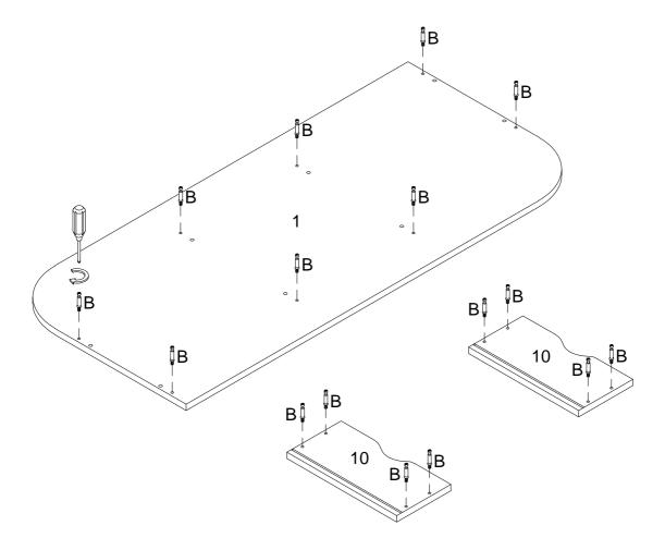
Secure cam bolt (B) into parts (1,10) with Philips head screwdriver as per diagram.
