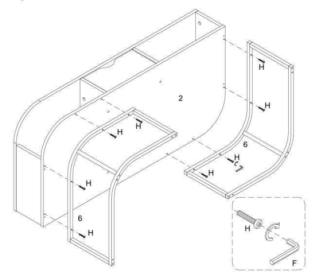
Using bolt (H) attach part (6) into part (2) with hex key (F) as per diagram.
