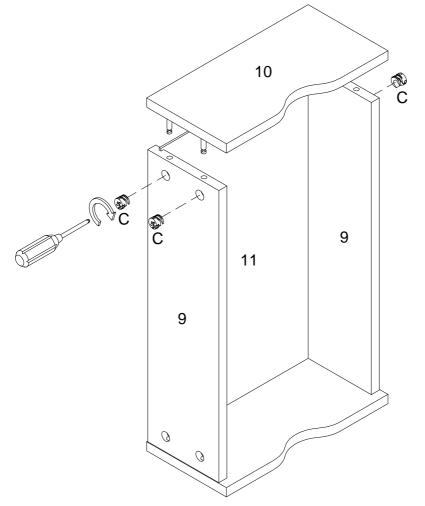
Using cam lock(C) attach part (10) to part (9) with Philips head screwdriver as per diagram.
