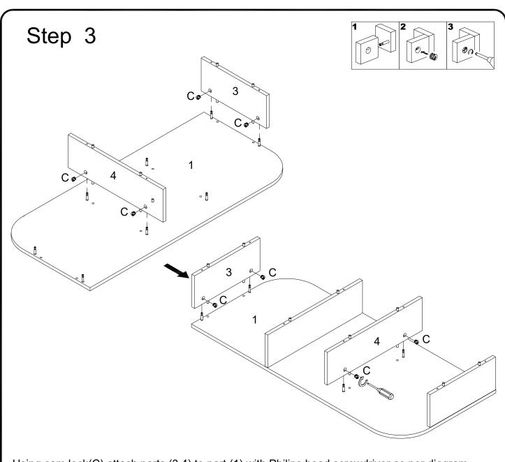
Using cam lock(C) attach parts (3,4) to part (1) with Philips head screwdriver as per diagram.
