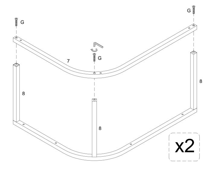
Using bolt (G) attach part (7) into part (8) with hex key (F) as per diagram.
