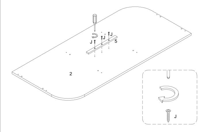
Using screw (J) attach part (5) to part (2) with Philips head screwdriver as per diagram.
