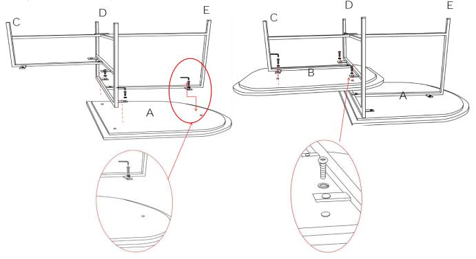
Tip A: Sometimes the Table will not balance because of an uneven floor surface the furniture rests on. In that case, try adjusting the levelers found on the bottom of each foot to aid in correcting.
