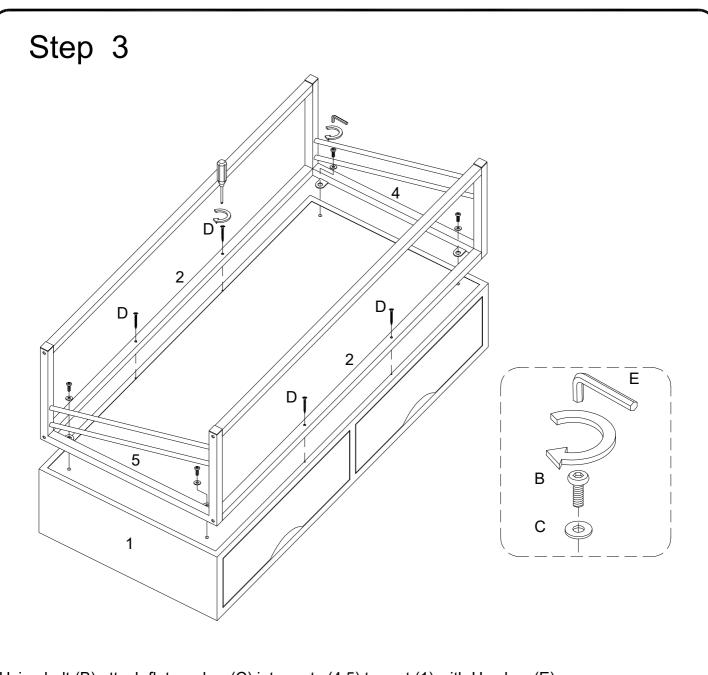
Using bolt (B) attach flat washer (C) into parts (4,5) to part (1) with Hex key (E), then using bolt (D) attach part (2) to part (1) with Philips head screwdriver as per diagram.
