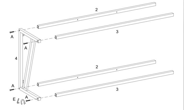
Using bolt (A) attach part (4) to parts (2,3) with Hex key (E) as per diagram.
