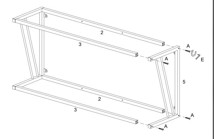
Using bolt (A) attach part (5) to parts (2,3) with Hex key (E) as per diagram.
