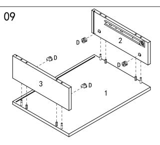
Put 4pc cam lock(D) inside the hole and fix drawer left and right panels with top panel.
