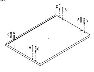
Screw 4 pc cam lock pin(C) on top panel(1), and insert 4pc wooden dowel(A).
