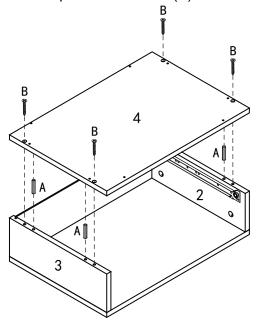
Insert 4pc wooden dowel on drawer right and left panels(2,3), and use 4pc screws(B) to fix bottom panel(4) to (2,3).
