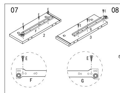
Use screw(E) to fix left drawer rail (F) on drawer left panel(2) and fix right drawer rail(G) on drawer right panel(3).
