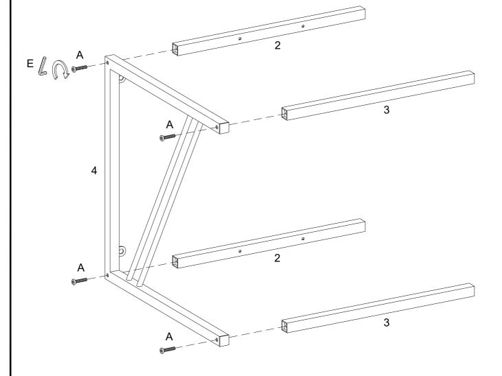
Using bolt (A) attach part (4) to parts (2,3) with Hex key (E) as per diagram.
