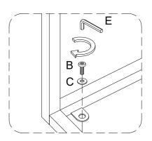
Using bolt (B) attach flat washer (C) into parts (4,5) to part (1) with Hex key (E), then using bolt (D) attach part (2) to part (1) with Philips head screwdriver as per diagram.
