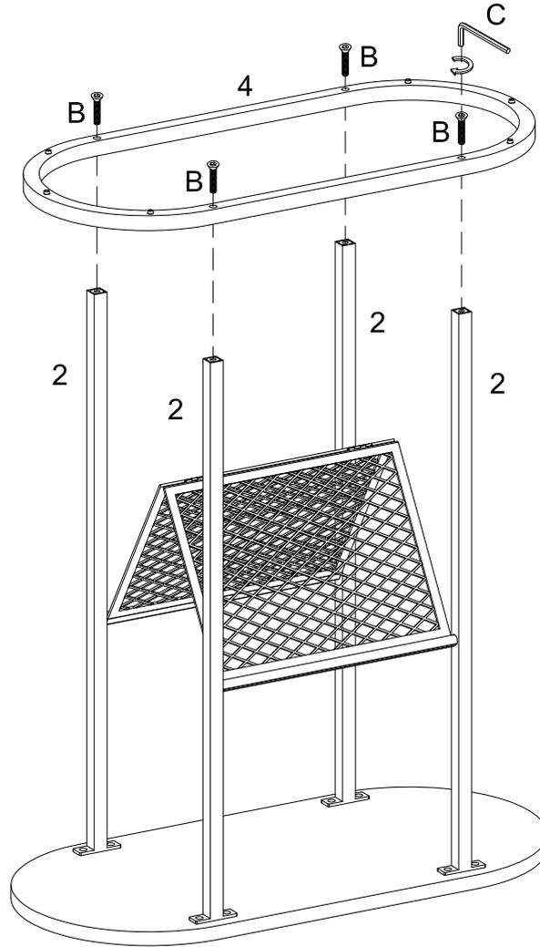
Using bolt (B) attach part (4) to part (2) with Hex key (C) as per diagram.
