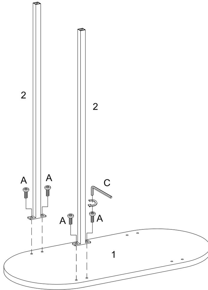
Using bolt(A) attach part (2) to part (1) with Hex key (C) as per diagram.
