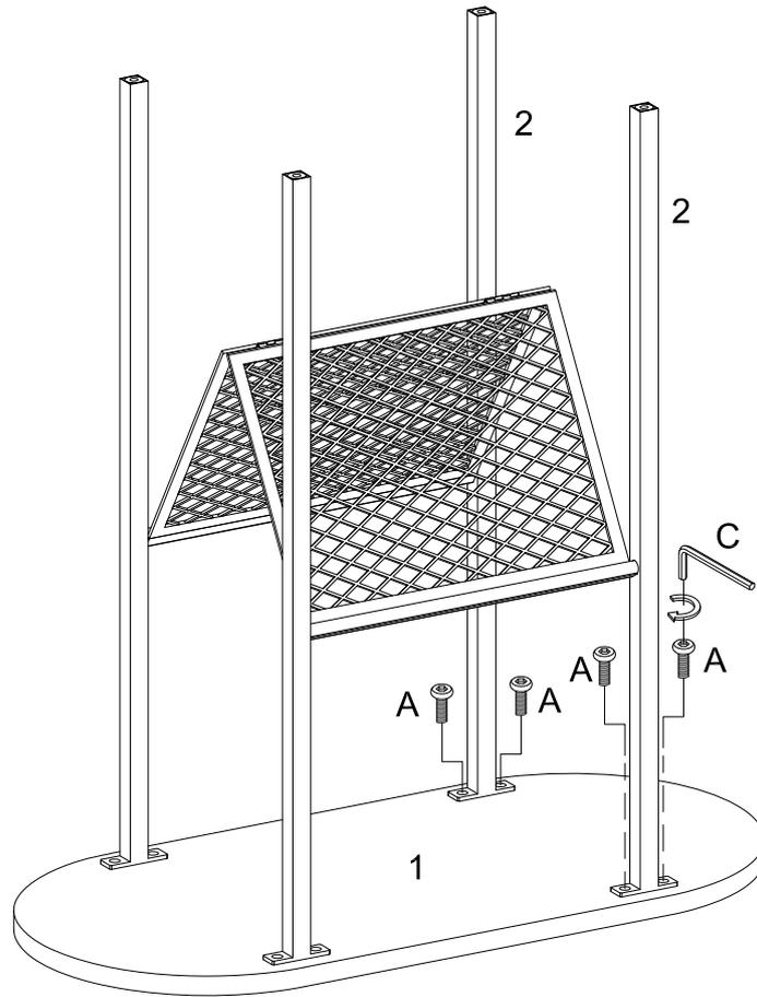
Using bolt (A) attach part (2) to part (1) with Hex key (C) as per diagram.
