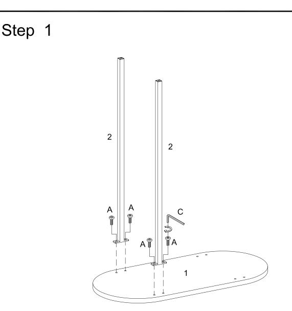
Using bolt(A) attach part (2) to part (1) with Hex key (C) as per diagram. Note : Do not fully tighten all the bolts .
