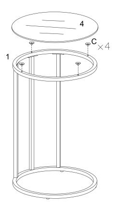
Insert rubber suction cups (C) into part (1), then place glass (4) on top of part (1) carefully.
