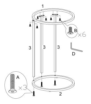
Attach part (3) to part (1) using bolt (B), and part (3) to part (2) using bolt (A) with hex key (D).
