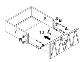
Turn the drawer upside down. Line up the holes on the outside pieces with the holes on the runners (GDR & GDL), secure to the drawer using screws (E).
