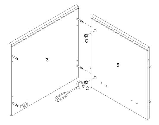
Using Cam lock(C) attach part (3) to part (5) with Philips head screwdriver as per diagram.
