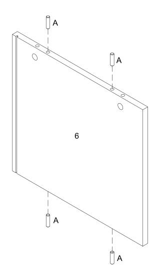
Insert wooden dowel (A) into parts (5,6) as per diagram.
