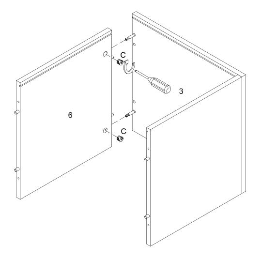
Using Cam lock(C) attach part (3) to part (6) with Philips head screwdriver as per diagram.
