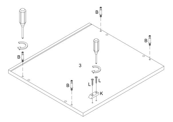
Secure cam bolt (B) into part (3),then using screw (L) attach Door stopper (K) to part (3) with Philips head screwdriver as per diagram.
