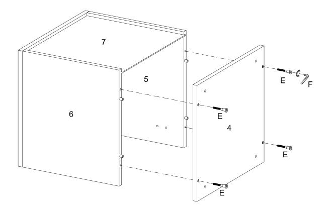
Using bolt (E) attach part (4) into parts (5,6,7) with hex key (F) as per diagram.
