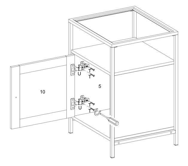
Using screw (T) attach Europe hinge (U) to part (5) with Philips head screwdriver as per diagram.
