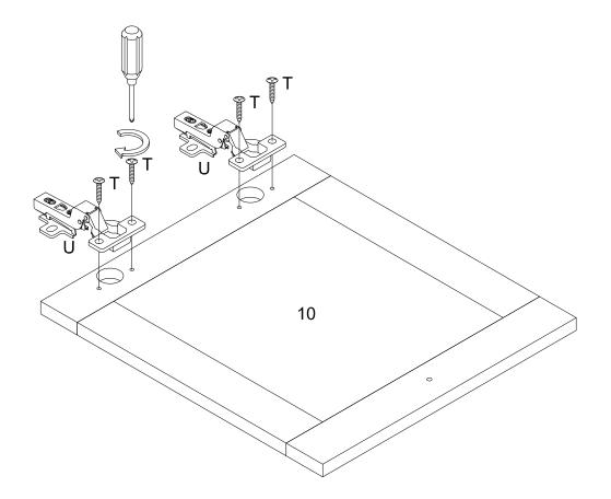
Using screw (T) attach Europe hinge (U) to part (10) with Philips head screwdriver as per diagram.
