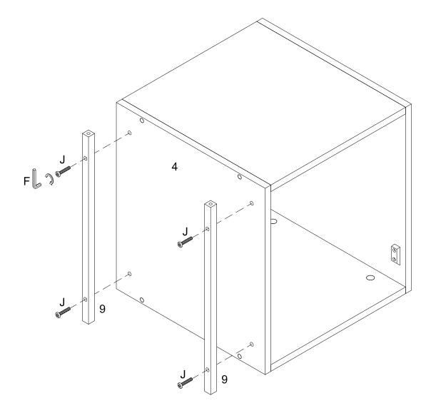
Using bolt (J) attach part (9) to part (4) with hex key (F) as per diagram. Note: Do not fully tighten all the bolts.
