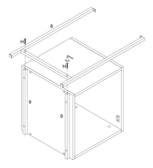
Using bolt (H) attach part (8) to part (9) with hex key (F) as per diagram.
