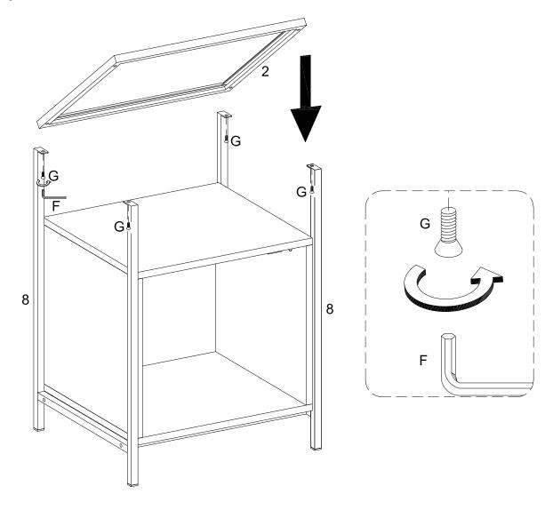
Using bolt (G) attach part (8) to part (2) with hex key (F) as per diagram.
