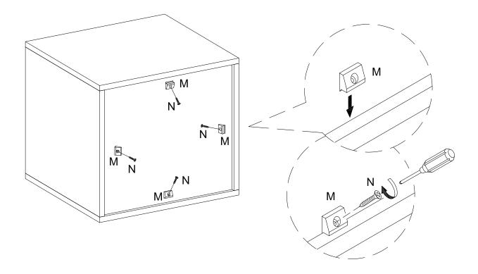
Using screw (N) secure plastic wedge (M) with Philips head screwdriver as per diagram.
