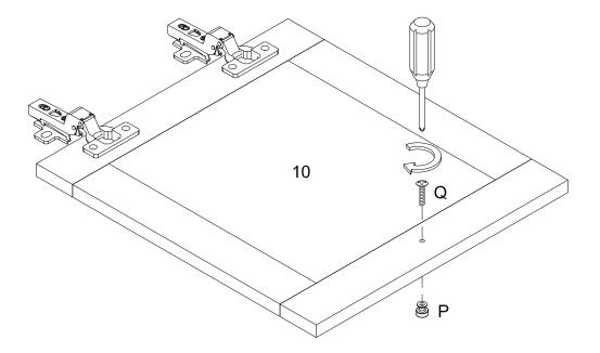
Using Handle bolt (Q) attach Handle (P) into part (10) with Philips head screwdriver as per diagram.
