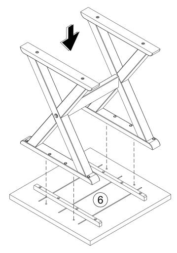
Step 7 Use Screw A to attach legs to part 6
