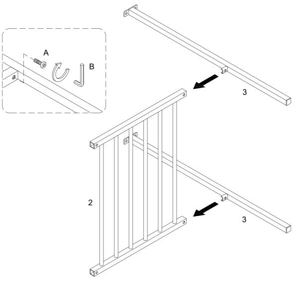
Attach part (3) to part (2) ,then using bolt (A) secure part (2) to part (3) with Hex key (B) as per diagram.
