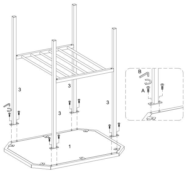
Using bolt (A) attach part (3) to part (1) with Hex key (B) as per diagram. Note: Fully tighten all bolts.
