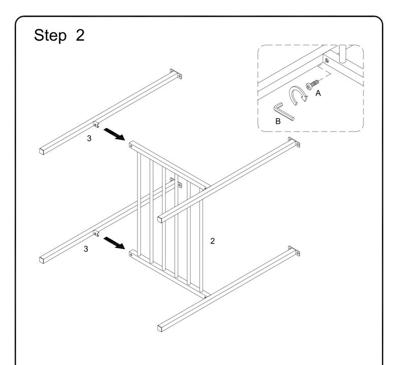
Attach part (3) to part (2) ,then using bolt (A) secure part (2) to part (3) with Hex key (B) as per diagram.
