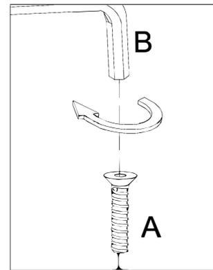
Using bolt (A) attach parts (3) into part (1) with hex key (B) as per diagram. Then fully tighten all the bolts.
