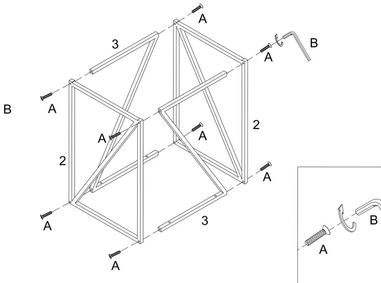
Using bolt (A) attach part (3) into part (2) with hex key (B) as per diagram.
