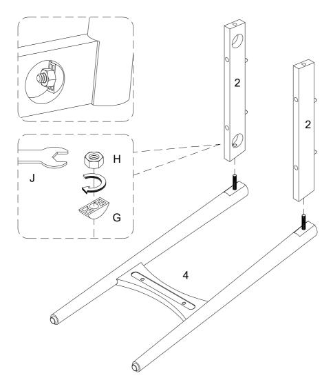
Using washer (G) and Nut (H) secure part (2) into part (4) with Wrench (J) as per diagram.
