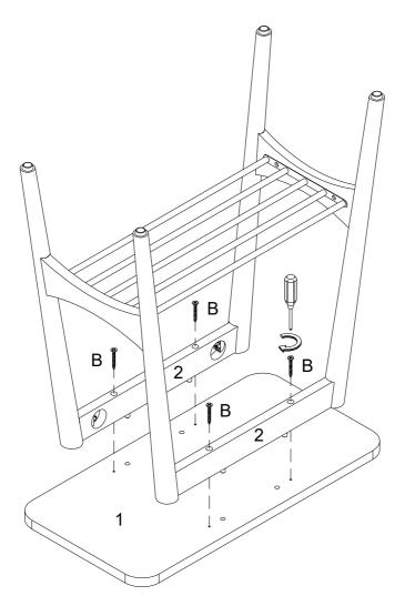
Using Flat head screw(B) secure part (2) to part (1) with Philips head screwdriver as per diagram. Note: Fully tighten all bolts.
