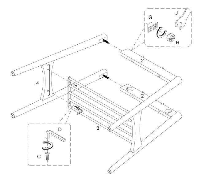
Using washer (G) and Nut (H) secure part (2) into part (4) with Wrench (J) ,then using bolt (C) attach part (3) to part (4) with Hex key (D) as per diagram.
