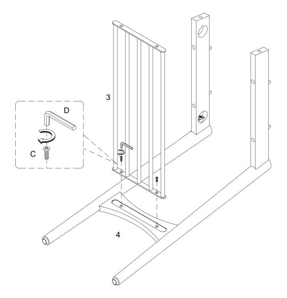
Using bolt (C) attach part (3) to part (4) with Hex key (D) as per diagram. Note:Do not fully tighten all bolts.
