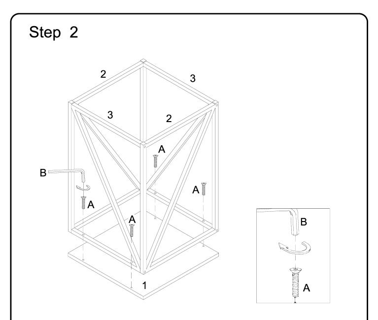
Using bolt (A) attach parts (3) into part (1) with hex key (B) as per diagram. Then fully tighten all the bolts.
