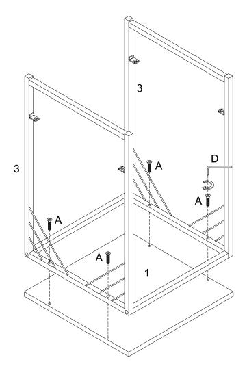
Using bolt (A) attach part (3) into part (1) with hex key (D) as per diagram.
