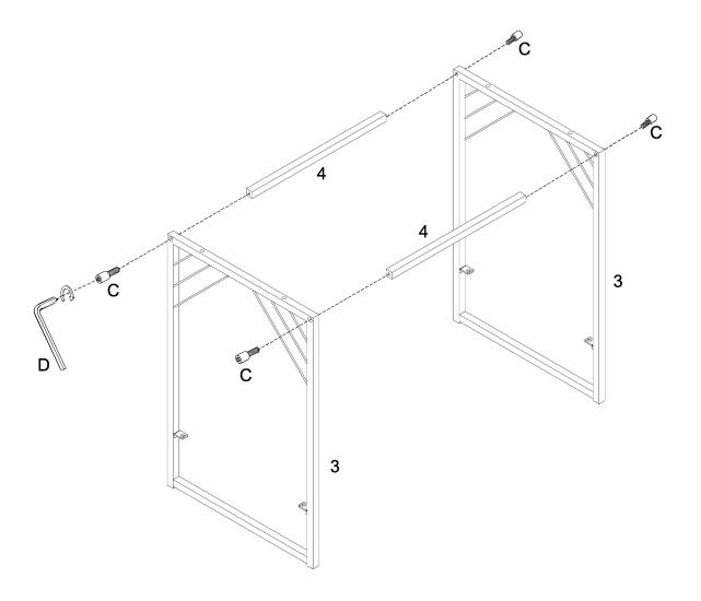
Using bolt (C) attach part (4) into part (3) with hex key (D) as per diagram. Note: do not fully tighten all the bolt.
