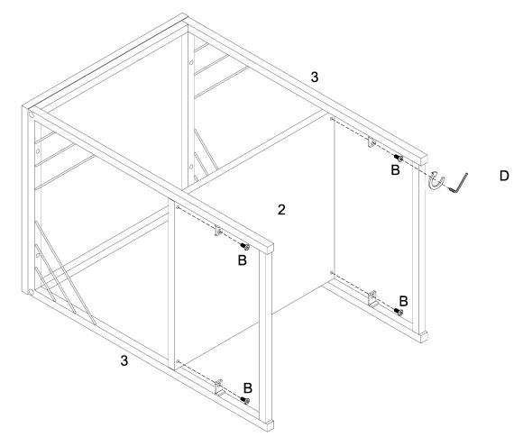
Using bolt (B) attach part (2) into part (3) with hex key (D) as per diagram. Then fully tighten all the bolts.
